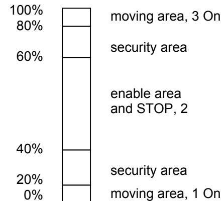
→ switching power on while DMX IN is active and the value is in the enable area, the STOP relay is triggered once. Switching power on while DMX IN is not present or the value is outside the enable area – nothing happens.
